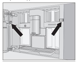
2 TX20 (25 mm) screws are supplied with the appliance.
