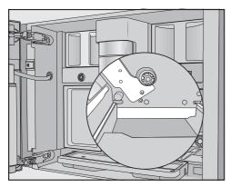
Clean the niche of the brew unit with a damp, clean cloth. Clean the areas marked in white in the illustration, e.g. around the drive shaft, especially well.
