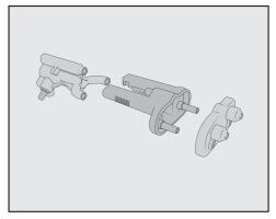
Dismantle the dispensing unit into 3 pieces: disconnect the Y-shaped piece, the dispensing spouts and the holder from one another.
