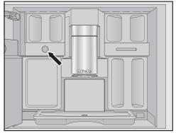
The milk valve is located under the bean container on the left-hand side.
