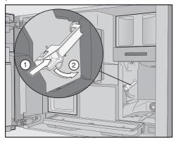
■ Press the button under the handle of the brew unit ① and, whilst doing so, turn the handle to the rear ②. **Useful tip:** If the handle of the brew unit cannot be turned, press firmly on the side of the brew unit.
