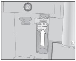
■ Insert the plug in place of the cartridge.
