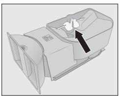
Do not remove the components which assist the flow of beans (see arrow).
