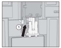
Release the milk pipework from the dispensing unit: to do this, pull the lug 1 to the left.
