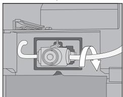
**Useful tip:** If necessary, turn the milk pipework on the right connecting piece towards the back.
