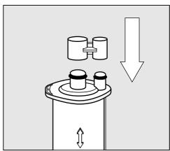
**Useful tip:** You can seal the descaling cartridge with the cap located on the cylinder of the cartridge. The cap can easily be released by snapping it off.
