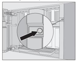
There is a red silicone plug inside the screw hole which secures the appliance door during transport to prevent transport damage.
