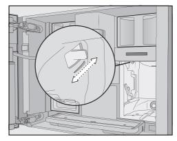
Push the slide control one setting to the front (for finer grinding) or to the back (for coarser grinding).
