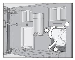
■ Pull the brew unit to the side ① first and then pull out to the front ②. Tilt the brew unit forward ③.
