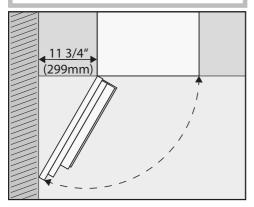
**Tip:** If a gap of at least 11 ¾" (299 mm) is maintained between the wall and the coffee machine, you will be able to open the appliance door wider, making the machine easier to use. For instance, it will be easier to remove the left-hand bean container.
