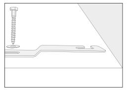
■ Install the fixing bracket with the hexagonal screws and the washers.
