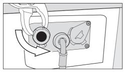
Unscrew the stopper from the hot water valve. Screw on the hot water hose.
