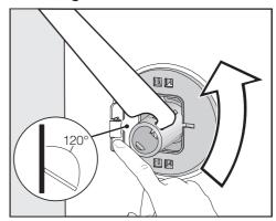
■ Push the cover out and turn the transit bar 90° using the open spanner supplied.
