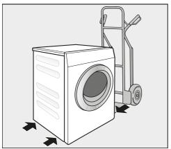
If transporting the washing machine with a hand trolley, make sure only its left or right side is resting on the trolley.
