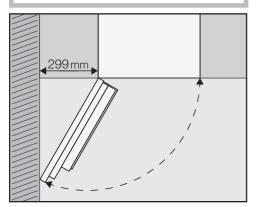
**Tip:** If a gap of at least 299 mm is maintained between the wall and the coffee machine, you will be able to open the appliance door wider, making the machine easier to use. For instance, it will be easier to remove the left-hand bean container. To install the machine, you will need a TX 20 screwdriver.
