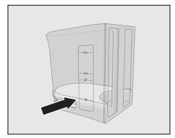
■ Fill the water container with lukewarm water up to the ///\\ mark and stir the solution.
