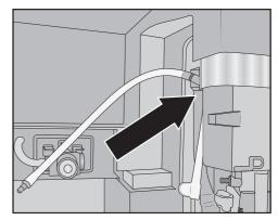
Connect together the angular moulded hose and longer milk pipework. Start by attaching the moulded hose to the top of the central spout. The black connecting piece should be pointing to the rear.
