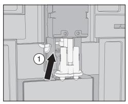
Detach the milk pipework from the dispensing unit as follows: pull the opening tag ① to the left.
