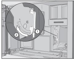
Press the button under the handle of the brew unit ① and, whilst doing so, turn the handle forwards ②.
