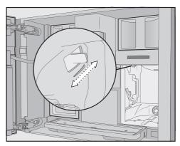
Push the slide control exactly 1 setting forwards (for finer grinding) or one setting backwards (for coarser grinding).
