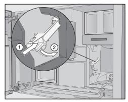
Press the button under the handle of the brew unit ① and, whilst doing so, turn the handle backwards ②.
