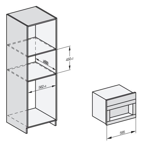
The appliance can be combined with other Miele built-in appliances. If the coffee machine is to be built in above another appliance, there must be a full-width, closed intermediate shelf between them. If the appliance is to be combined with a Gourmet drawer/built-in vacuum drawer, no intermediate shelf is required in between.
