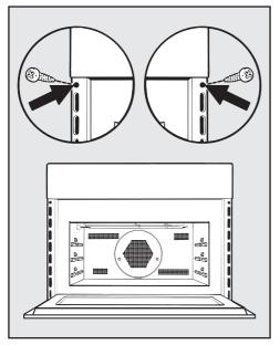
Open the door and use the screws supplied to secure the oven to the side walls of the housing unit.
