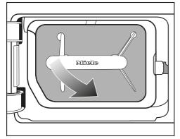
1 Use the handle to pull out the lint filter at an angle forward and to the right.
