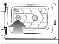
2 Then press on the left handle until the filter insert is secured in position.
