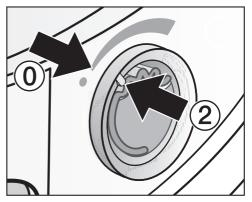
■ Turn the outer ring counterclockwise until marker ② is in position ①.
