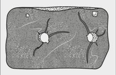
Lint will blow into the heat exchanger through cracks and tears and will cause obstruction.
