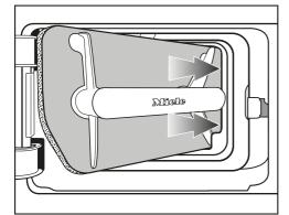
① Use the handle on the right to slide the lint filter at an angle behind the edge.
