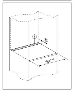
■ Create a cut-out ① in the intermediate shelf where the steam oven is to be placed.
