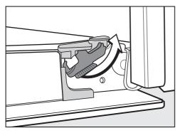
Release the locking clamps by turning them as far as they will go. The oven could become damaged if you incorrectly remove the door.
