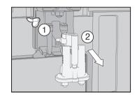
Detach the milk pipework from the dispensing unit 1. Pull the dispensing unit down to remove it 2.
