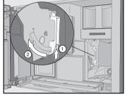
Press the button under the handle of the brew unit (1) and, whilst doing so, turn the handle forwards 2.
