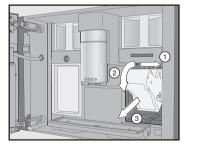
Pull the brew unit sideways ① and then tilt it forwards 2. Pull the brew unit forwards to remove it ③.
