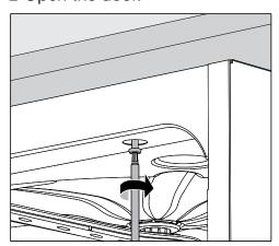
■ Screw the machine to the continuous countertop through the holes in the front trim on the left and right.
