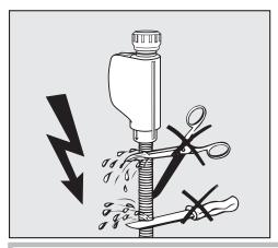
Do **not** shorten or otherwise damage the inlet hoses supplied with the machine.
