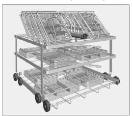
An injector manifold with silicone hoses with Luer Lock connectors is located on the upper level. Trays and mesh trays for ophthalmological OR sets with integrated injector manifolds can be connected to this manifold.
