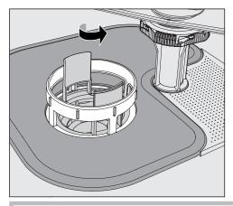
⚠ Danger of injury from glass shards, needles etc. which are retained in the filters.
