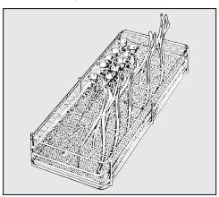
■ To ensure coverage of all surfaces by the wash fluid please open specula and place in the insert.
