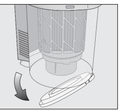
The dust container flap will open and the dust will fall out.
