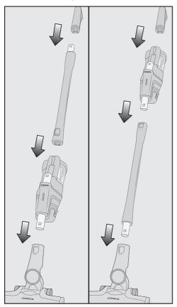
You can place the suction tube either above or below the PowerUnit.
