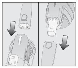
Slide the suction tube along the guide line on the dust container handle and down onto the PowerUnit connector from above until it audibly clicks into place (left image detail).
