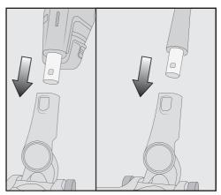
Push the connector into the Electrobrush from above until it audibly clicks into place.
