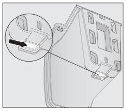
Press the release catch at the bottom of the wall bracket.
