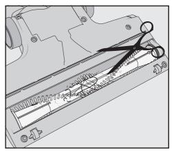
Cut any threads or hairs that have wound themselves around the roller brush with a pair of scissors. To guide the scissors, move along the guide track on the roller brush. Then run the vacuum cleaner to vacuum up the cut threads and hairs.
