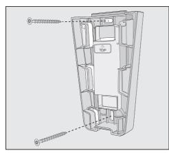
Attach the mounting plate to the wall.
