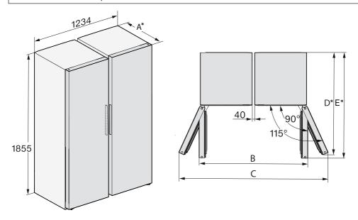
\* Dimensions without wall spacers fitted. Appliance depth is increased by 15 mm with the wall spacers supplied fitted.
