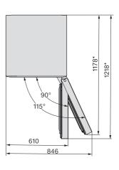
\* Dimensions without wall spacers fitted. Appliance depth is increased by 15 mm with the wall spacers supplied fitted.
