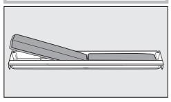
Remove both charcoal filters and place the new filters with the surrounding edge pointing downwards in the holder.
