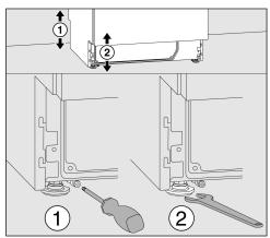
The front machine feet can be adjusted with an open spanner (spanner size 13); the rear ones with a T20 Torx screw.
