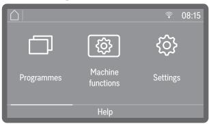
If the machine has been networked, a symbol for the available interface is shown at the top of the display.  $\ \$  stands for a WiFi connection,  $\ \$  for a wired LAN connection. If the machine cannot establish a WiFi connection with the router, the symbol will be shown with a cross through it  $\ \ \$ .
