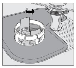
■ Loosen the microfine filter by turning it in the direction of the arrow and remove it together with the coarse filter.
