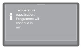
If the temperature inside the wash cabinet is more than 60 °C at this point, the pressure is equalised first. Then the programme continues.
