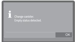
System messages are indicated by the information symbol 1. These give information about current processes and the status of the machine. If there is more than one system message, they are shown one after the other and — depending on the message — must be processed or acknowledged individually.
