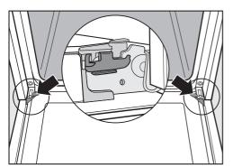
The oven door is connected to the door hinges by retainers.
