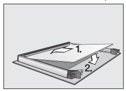
■ Refit the middle pane in such a way that the material number is legible (not reversed).
