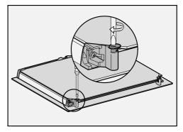
Use a flat-head screwdriver to flip the two glass pane retainers outwards.
