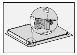
Use a flat-head screwdriver to flip the two glass pane retainers inwards.
