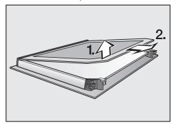
■ **Gently** lift the inner pane up and out of the plastic strip.
