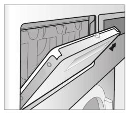
If the drip channel and associated drain connection are blocked, clean them.
