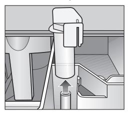
■ Remove the siphon. Clean the siphon with hot water and reinsert it.
