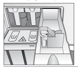
Do not fill the  $\frak{\$}$  compartments above the level marker with liquid agents.
