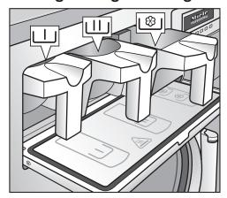
■ For standard wash programs, add powder detergent for the main wash to the Ш compartment and if desired, add detergent for a pre-wash to the Ш compartment. Add fabric softener to the front of the 🕮 compartment.
