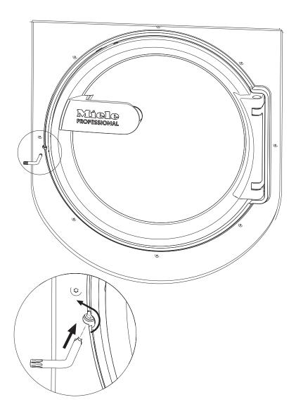
■ Turn the release element with a T 40 Torx wrench two whole revolutions counter-clockwise (left).
