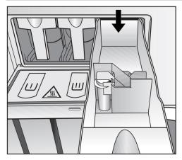
Liquid bleaching agents must only be dispensed through the designated dispenser drawer compartment. Only then it is ensured that the agent is added in to the second rinse cycle automatically. Liquid bleaching agents should only be used on colored textiles which have a wash care label stating that they are suitable for bleaching.
