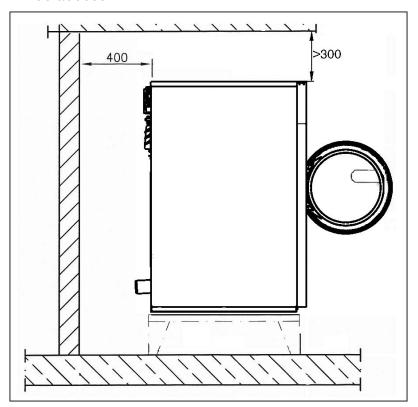
Minimum safety distance to the wall approx.15 3/4" (400 mm) to allow for maintenance.
