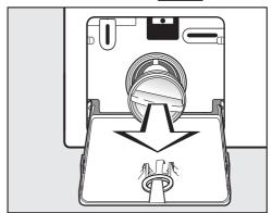
■ Remove the drain filter completely.
