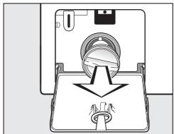
■ Remove the drain filter completely.
