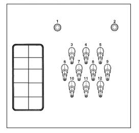
Dispenser pump connections on the back of the machine
