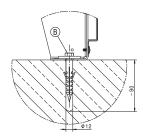
Dimensions in millimetres (B) screw / anchor point
