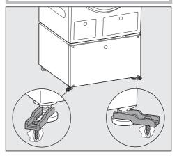
Anchor the base to the floor with the tensioning strips provided.
