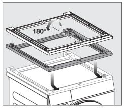
■ Turn the stacking kit the right way up and place it on the washing machine lid.
