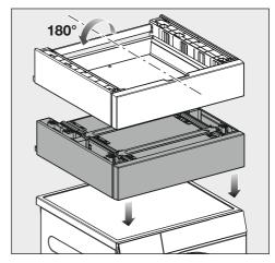
■ Turn the stacking kit the right way up and place it on the washing machine lid.
