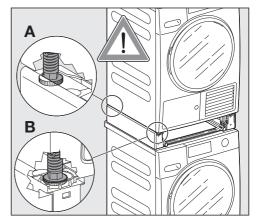
The tumble dryer feet are positioned securely in the stacking kit.
