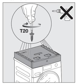
■ Carefully tighten the screws by hand. Do not overtighten the screws.
