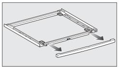
Remove the screen from the stacking kit
