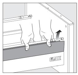
■ Place the bottom of the panels in position and press the panels inward at the top.
