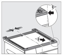
■ Use the front edge of the washing machine lid and the edges of the stacking kit for this purpose.
