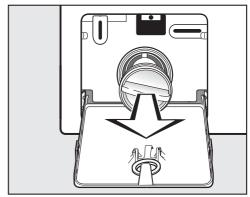
■ Remove the drain filter completely.
