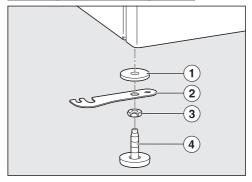
■ Install the connecting pieces together with the feet that have been removed.
