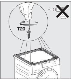
■ Carefully screw the stacking kit onto the washing machine lid by hand. Do not overtighten the screws.
