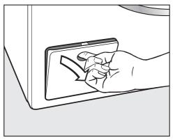
Open the access panel for the drain pump.
