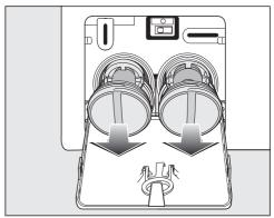
■ Remove the filters completely.
