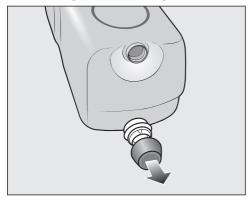
Remove the cover cap from the cartridge.
