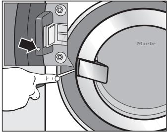
4 mm blade) into the opening next to the door lock and use it to release the catch. Turning it slightly in an anticlockwise direction should release the door.
