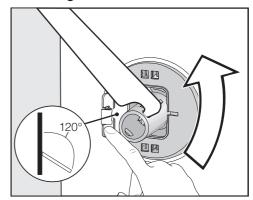
■ Push the cover out and turn the transit bar 90° using the open spanner supplied.
