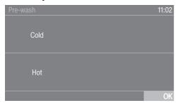
Touch the cold sensor control if the washing machine is only connected to a cold water supply, or touch hot if the washing machine is connected to cold and hot water.
