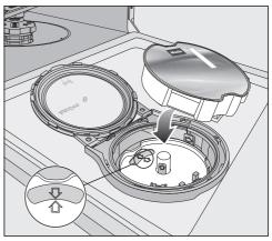
If the arrows in the PowerDisk holder and in the viewing window are not pointing towards each other, remove the PowerDisk holder.
