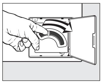
■ Push the emergency drain lever downwards (see illustration) and hold until no more water runs out.
