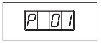
The letter " P " (code for programming level) will appear on the left hand side of the display. The " 01" on the right of the display shows the first input position.
