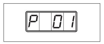
The letter " P " (code for programming level) will appear on the left hand side of the display, and the first input position will show on the right hand side of the display.
