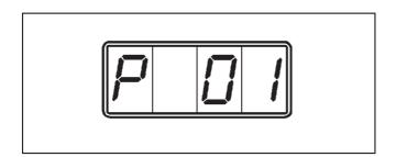
The letter " P " will appear on the left hand side of the display. The " D1 " on the right of the display shows the first input position.
