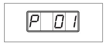
The letter " P " (code for programming level) will appear on the left hand side of the display. The " 01" on the right of the display shows the first input position.
