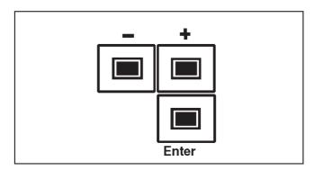
■ Press and release the " Enter " button 4 times within 5 seconds .
