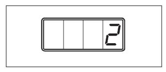
■ Press the " + " or " - " button until the required option (1,2,3,4 ...9999) shows in the display (e.g. " 2" for timed operation).
