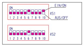
or 10 (4S1), depending on coin tester, upwards. Use a suitable tool, e.g. a ball-point pen to do this.
