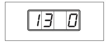
The " " on the right of the display shows that the channel is " **barred** ".
