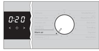
■ Touch the < or > sensor control until the required duration lights up.
