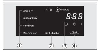
The 1-4 sensor controls react to fingertip contact. If a sensor control is illuminated, it can be selected.
