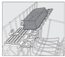
■ Secure light items to the MultiClips.
