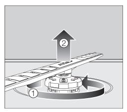
■ Rotate the screw connection of the lower spray arm anti-clockwise ① and pull the spray arm upwards to remove ②.
