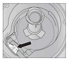
The drain pump (see arrow) is underneath the cover.
