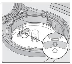
Put the holder back into place so that the arrows in the PowerDisk holder and in the viewing window point towards each other. The holder must lie flat. The AutoDos lid must close tightly so that the detergent powder does not get wet and clump together.
