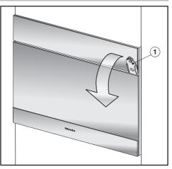
Insert the door tool ① supplied about 1 1/2" (3 cm) into the gap between the door and the control panel on the right-hand side and then pull the door open. Risk of injury caused by hot surfaces and food.
