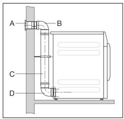
A Wall pipe, with suitable louvre. We recommend fitting a 90° downward facing elbow
