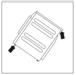
Carry the tumble dryer by the front feet and by the lid where it protrudes at the back of the appliance.
