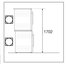
2 Miele tumble dryers can be installed as a dryer stack. A stacking kit\* is needed for this purpose. This must be fitted by a Miele authorised technician.
