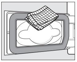
Use a damp cleaning cloth to remove any fluff. Make sure that you do not damage the rubber seal when doing this.
