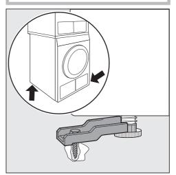
Secure 2 feet to the tumble dryer <u>diagonally at the front and rear</u> or <u>only at the rear</u>.
