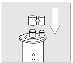
■ Seal the cartridge with the cap.
