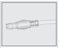
If you have released the connecting piece from the milk pipework: when reassembling, ensure that the smaller, thinner end of the connecting piece is pushed into the hose.
