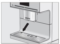
■ Remove the protective foil from the drip tray cover and place the drip tray cover into the lower panel.
