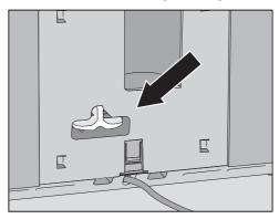
■ Fit the plug instead of the descaling cartridge.
