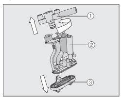
■ Twist off the upper section ① with the holder for the milk tube. Pull the component off. Then pull the Y-shaped piece ② off. Remove the dispensing spouts ③.
