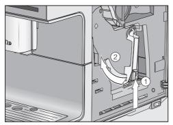
■ Press and hold the button under the brew unit handle ① and, whilst doing so, turn the handle to the left ②.
