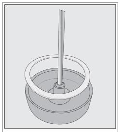
If necessary, you can remove the connecting piece and sealing ring from the milk flask lid. Once you have removed the stainless steel tube, the connecting piece is easy to push out from the inside of the lid.
