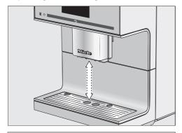
The height of the central spout with cup rim sensor **cannot** be manually adjusted.
