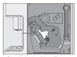
Clean the interior of the coffee machine. Make sure that the areas highlighted (in white) in the illustration are cleaned especially well.
