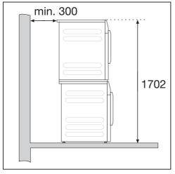
The washing machine can be installed as a washer-dryer stack together with a Miele tumble dryer. This requires a Miele washer-dryer stacking kit which can be purchased separately. A Installing the washer-dryer stack on a Miele plinth is not permitted.
