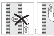
If the exhaust air is to be ducted into a flue, the ducting must be directed in the flow direction of the flue.
