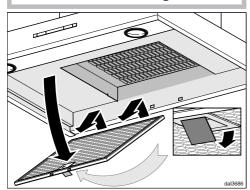
■ To take out a grease filter, release the locking clip on the filter, lower the filter approx. 45°, unhook it at the back and remove it.
