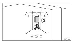
In recirculation mode, the silencer needs to be positioned between the exhaust socket and the directional unit ②. Check that there is sufficient space.
