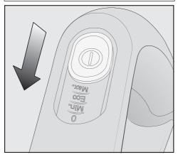
■ Press the On/Off switch on the Comfort handle (1).
