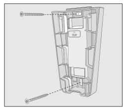
Attach the mounting plate to the wall.
