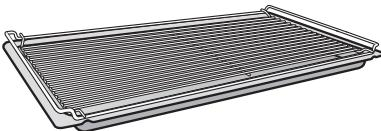
If you are using the universal tray with the rack on top, insert the tray between the rails of the shelf runners and the rack will automatically slide in above them.
