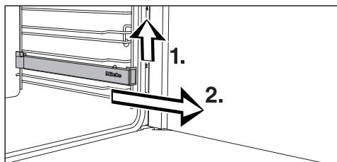
■ Remove the FlexiClip telescopic runner by raising it at the front (1.) and then pulling it forwards along the rail of the shelf level and out (2.).
