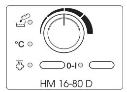
The **I-0** "On-Off" button is used for switching the ironer on and off.
