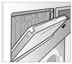
If the drip channel and associated drain connection are blocked, clean them
