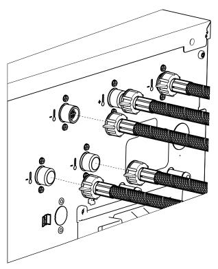
Before attaching the inlet hoses to the machine, the filters and seals included in the accessory pack must be inserted.
