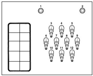
Connections **1** and **2** are provided for viscous agents. These connectors are sealed and need to be drilled open using an 8 mm drill bit.
