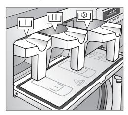
■ For standard wash programs, add powder detergent for the main wash to the Ш compartment and if desired, add detergent for a pre-wash to the U compartment. Add fabric softener to the front of the 🖹 compartment.
