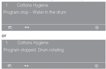
**Tip:** To open the door, press the "Water drain" function button or select the "Extra Spin" program and press the "START" button.
