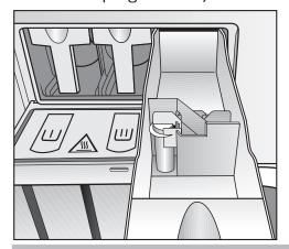
Do not fill the  $\fill \$  compartments above the level marker with liquid agents.
