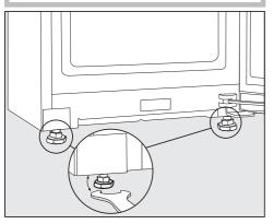
■ To align the refrigeration appliance, adjust the front feet using a spirit level and the spanner supplied.
