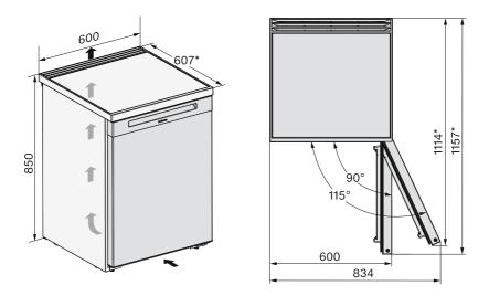
$<sup>^{\</sup>star}$  Dimensions without wall spacers fitted. Appliance depth is increased by 35 mm with the wall spacers supplied fitted.
