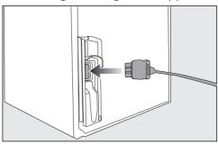
Insert the plug connector into the socket at the back of the refrigeration appliance.
