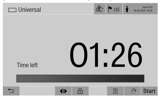
The pictogram of the load carrier and the selected reprocessing program are displayed in the header.
