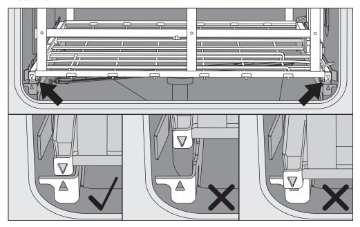
The markings on the load carrier ▼ and in the wash cabinet ▲ need to be flush with one another.
