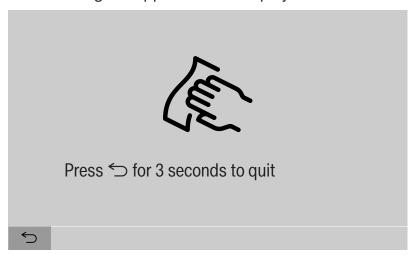
lacktriangle To unlock the machine display, hold the  $\circlearrowleft$  button for around 3 s.
