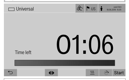
After selecting a program, the time left for the selected reprocessing program is displayed. If the Display time remaining parameter is not activated in the web interface, the display switches to the already elapsed Duration of the reprocessing program after program start.
