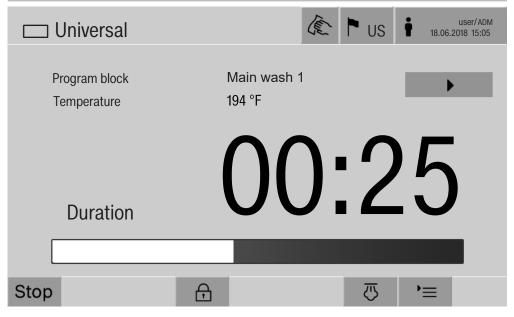
After the reprocessing program has started, an additional ▶ button is displayed next to the program phase. The ▶ button has two functions:
