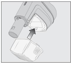
Push the battery along the guide lines until it audibly clicks into place in the PowerUnit.
