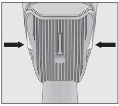
Press both release buttons at the side of the battery at the same time to remove the battery.
