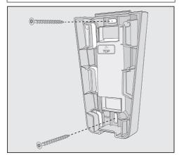
Attach the mounting plate to the wall.
