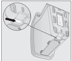
Press the release catch at the bottom of the wall bracket.
