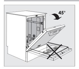
■ Open the door to an angle of around 45°. This ensures that the salt flows into the container more easily.
