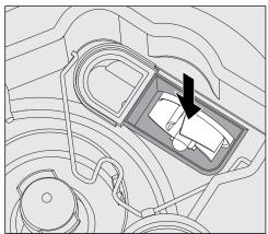
The drain pump impeller is situated under the non-return valve.
