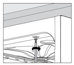
■ Remove the cover caps on the left and right. Screw the machine to the continuous worktop through the holes in the front trim. Then refit the cover caps.
