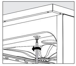
■ Remove the cover caps on the left and right and tighten the fixing screws. Then refit the cover caps.
