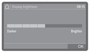
■ Adjust the brightness of the display and press *OK* to save the setting.
