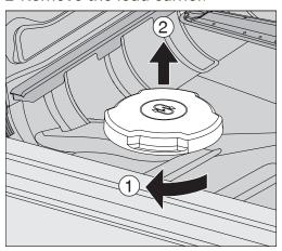
■ Turn the salt container cap in the direction of the arrow ① as far as it will go and pull the cap upwards ②.
