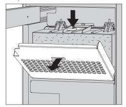
■ Loosen the filter grille and fold it downwards. Alternatively, you can also remove the grille.
