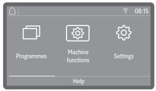
If the machine has been networked, a symbol for the available interface is shown at the top of the display.  $\widehat{\ast}$  stands for a WiFi connection,  $\mathsf{L}$  for a wired LAN connection. If the machine cannot establish a WiFi connection with the router, the symbol will be shown with a cross through it  $\widehat{\ast}$ .
