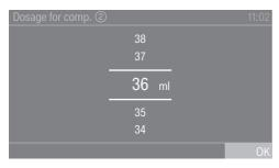
Confirm the preset value with the OK sensor control, or change the value.
