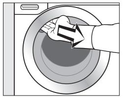
Reach under the recessed grip and pull the door open. Check the drum for pets or foreign objects before loading it with laundry.
