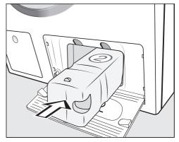
■ Push the UltraPhase 2 detergent cartridge into compartment 2 until it locks into position.
