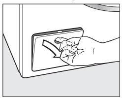
■ Open the drain pump access panel.
