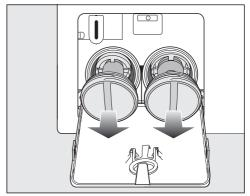
■ Remove the drain filters completely.
