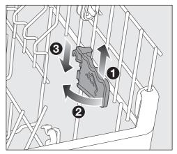
Slightly lift the XL-Assist 1, fold it out 2 and hook it back in the new position 3.
