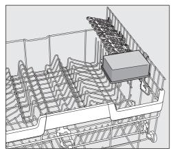
Secure light items to the MultiClips.
