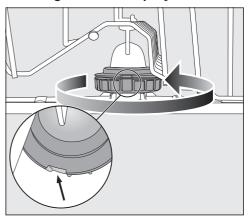
■ Replace the middle spray arm and turn the screw thread anti-clockwise (view from above) until it engages. Make sure that the recesses in the lock line up.
