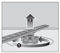
■ Rotate the screw thread of the lower spray arm anti-clockwise ① (view from above) and pull the spray arm upwards to remove ②.
