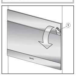
■ Insert the opener included with the appliance ① about 3 cm into the gap between the door and the control panel on the right-hand side and then pull the door open.
