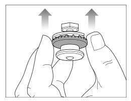
■ After cleaning, push the top heat/grill element back up using the outer ring of the pressure cap.
