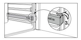
■ Then secure the FlexiClip runner to the lower rail of the shelf level (3.).
