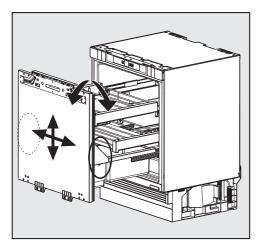
The adjustment options are located on the right-hand and left-hand sides underneath the bottle shelf on the inside of the door.
