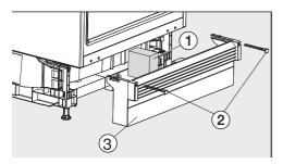
■ Replace the plinth panel with the ventilation grille ③, but do not fix it in place yet.
