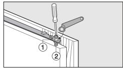
■ Whilst counterholding adjusting bolts ② with a screwdriver, tighten nuts ① on the appliance door with screwdriver.
