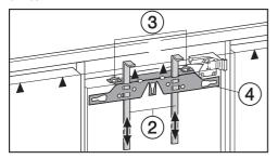
■ Undo the nuts ③ and take the fixing bracket ④ off together with the fitting aids ②.
