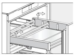
■ Holding the sides of the pull-out at the back, lift it up and then forwards and out.
