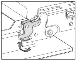
■ To relock the locking clamps, turn them back up to the horizontal position as far as they will go on both door hinges.
