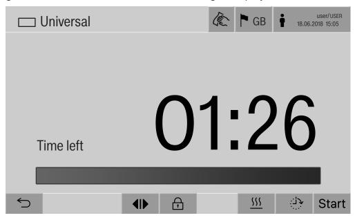
The pictogram of the load carrier and the selected reprocessing programme are displayed in the header.
