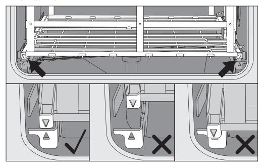
The markings on the load carrier ▼ and in the wash chamber ▲ must line up correctly.
