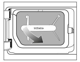
① Use the handle to pull out the lint filter at an angle forward and to the right.
