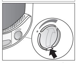
Push the tab down completely (see arrow) so that the socket is closed.
