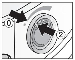
■ Turn the outer ring counterclockwise until marker ② is in position ①.
