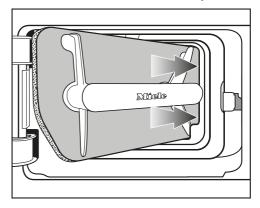
1 Use the handle on the right to slide the lint filter at an angle behind the edge.
