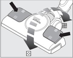
Clean hard flooring which is not susceptible to scratching, as well as flooring with gaps or deep crevices in it, with the brush protruding:
