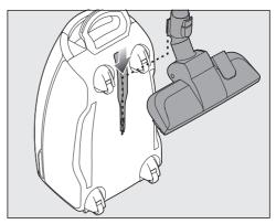
■ Slot the floorhead downwards into the parking attachment on the underside of the vacuum cleaner.
