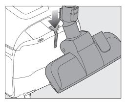
Slot the floorhead into the park system on the vacuum cleaner.
