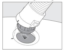
Insert the hose connector into the suction opening on the vacuum cleaner until it clicks into position. To do this, line up the guides on the two pieces.
