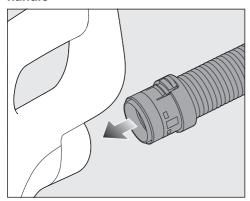
■ Fit the suction hose connector into the handle until it clicks into position.
