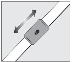
Grasp the release mechanism and adjust the telescopic tube to the required length.
