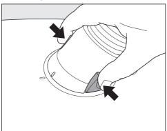
■ Press the release buttons at the side of the hose connector, and lift the hose from the suction opening.
