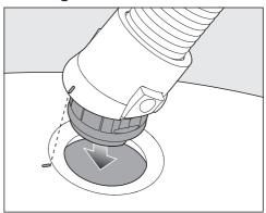
■ Insert the hose connector into the suction opening on the vacuum cleaner until it clicks into position. To do this, line up the guides on the two pieces.
