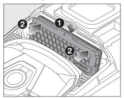
■ Insert the new exhaust filter downwards, making sure it goes in properly, then press it backwards on both sides until it clicks into place.
