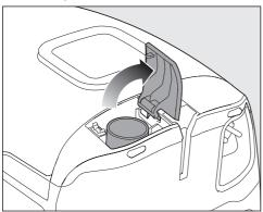
■ Press the release button on the accessories compartment.
