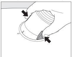
Press the release buttons at the side of the hose connector and pull the hose out of the suction opening.
