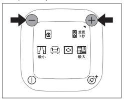
■ Press the + foot switch to select a higher suction power level.
