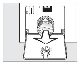
■ Remove the drain filter completely.
