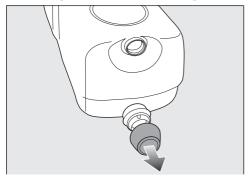
Remove the cover cap from the TwinDos cartridge.
