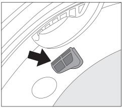
■ Remove the fluff with your finger. Do not use any sharp or pointed tools to do this.
