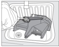
Clean the fabric conditioner channel using a bottle brush and warm water.
