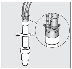
■ Insert the drain adapter into the plastic drain pipe.
