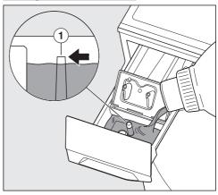
■ Add fabric conditioner or liquid starch to the % compartment. **Do not exceed the maximum level mark** ①.
