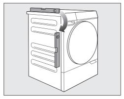
■ Use a spirit level to check the washing machine is standing level.
